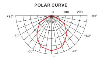
Intensity Distribution in cd/klm Ratio of Distance to Height: 2.5 Voltage and Frequency : 90V~260V AC 50/60HZ
